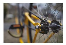
Bike spokes are "a key role in the transferring of the power from your legs to the rim to make the bike go. Enormous force gets applied to the hub of a rear wheel by the chain and gearing when you pedal down hard, and together the spokes carry the power that has gone from your legs to the chain then out to the wheel. That force driving the bike forward gets distributed among many spokes in a properly aligned wheel,
